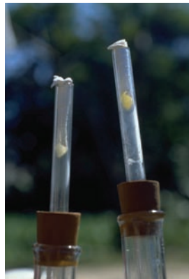
Litmus paper used to test well water for the presence of arsenic
